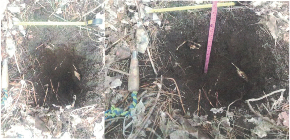
Plates B14 & B15: Sample Test Pit Stratigraphy in Forest Area of Property; Planview & Profile (yellow surface hand tape @30cm)
